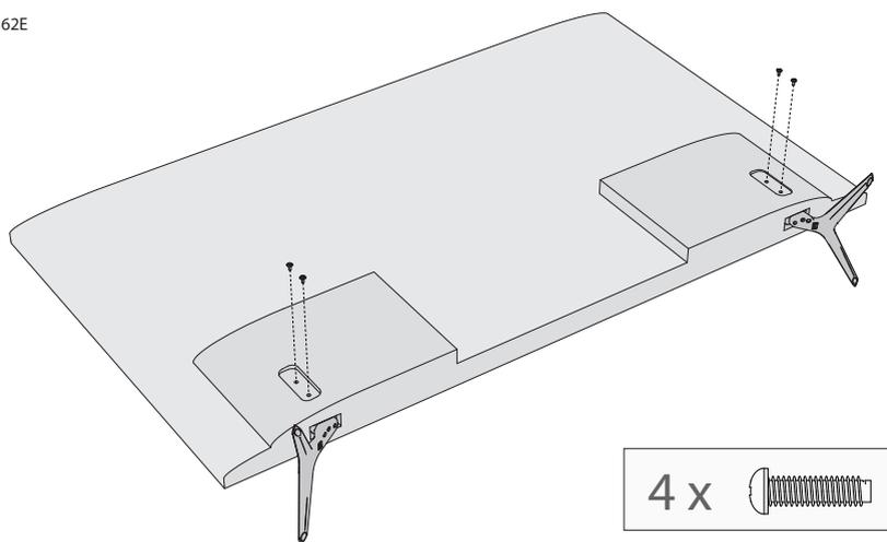
**English:** To assemble the base stand to the TV you will need a cross head screwdriver. To avoid damage to the TV screen during assembly ensure the TV is placed on a soft flat surface with the LCD screen facing downwards.
